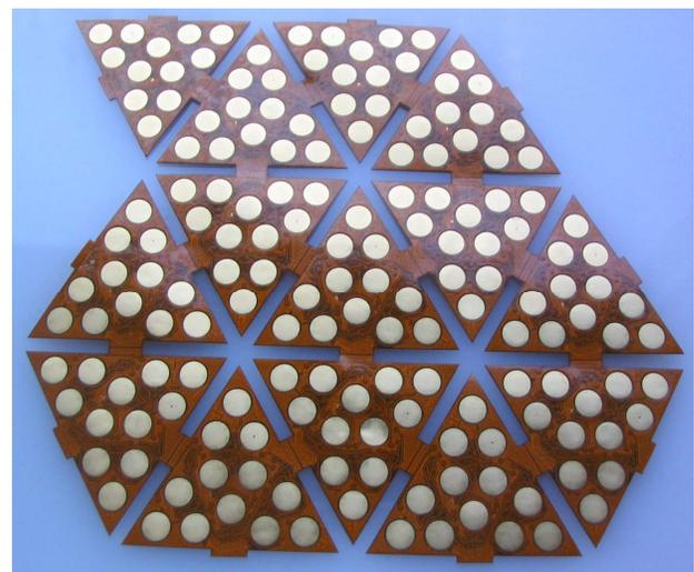
Fig. 4. 16 triangles interconnected on a flexible PCB.
