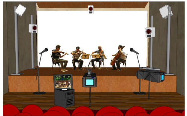
Figure 5: The multimodal setup for the experiment at Casa Paganini - InfoMus: (a) motion capture, (b) frontal videocamera, (c) videocamera for individual violinist, (d) environmental microphones. Each musician wear markers for motion capture and EMG on the right arm. Piezoelectric microphones are in the body of the violin for individual measurements.
